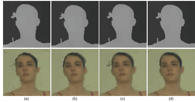
Fig. 6. Sample frames of the reconstructed depth map and rendered view for the Ballet sequence obtained by different in-loop filters: (a) H.264/AVC Deblocking filter, (b) Boundary reconstruction filter [7], (c) Trilateral filter [8], (d) Proposed in-loop filter.
