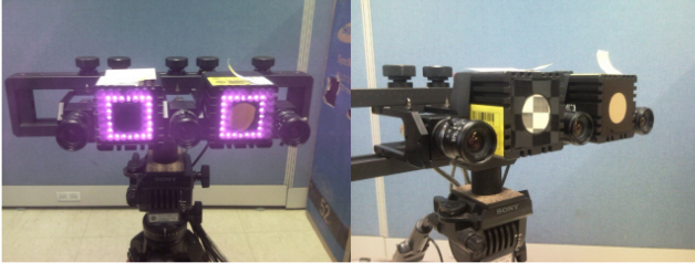
Fig. 1. Multiview color-plus-depth acquisition system: a hybrid structure with two ToF depth sensors and three color cameras.
