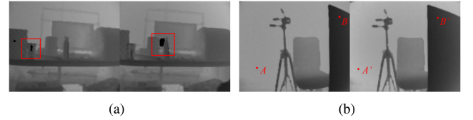
Fig. 6. Problems of the depth maps obtained from multiple depth sensors. (a) Unreliable depth acquisition. (b) Different depth values at the same world point.
