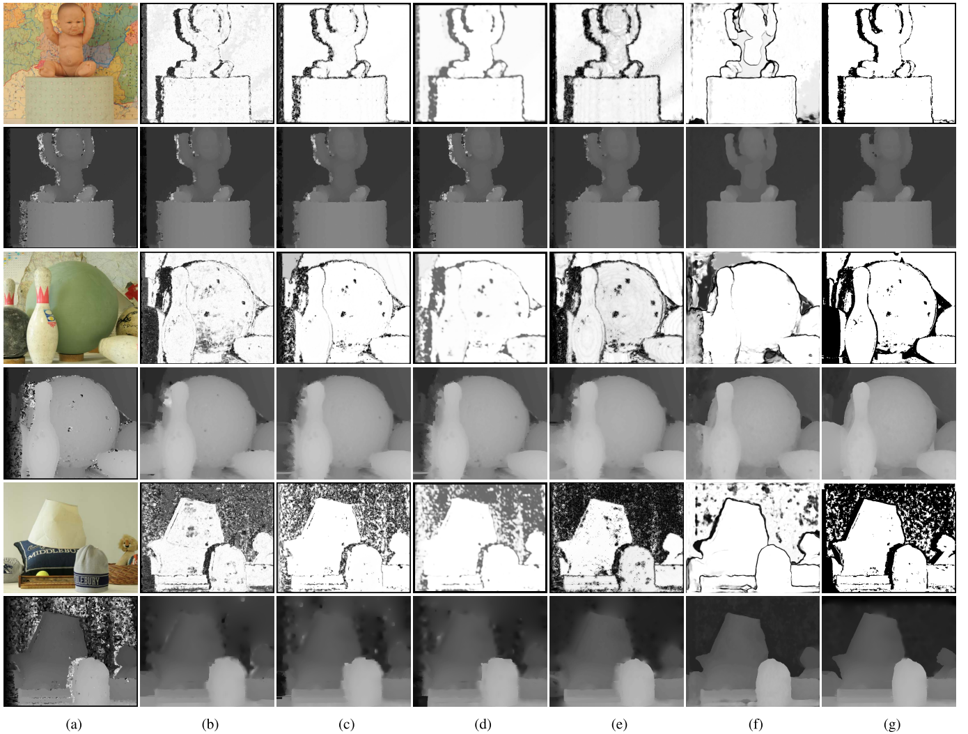
Fig. 12. The confidence and refined disparity maps on MID 2006 dataset [39] using MC-CNN+mod. (1st and 2nd rows), +GCPs (3rd and 4th rows), and +AGCPs (5th and 6th rows) (a) Color images and initial disparity maps, refined disparity maps with confidence maps estimated by (b) Haeusler et al. [23], (c) Poggi et al. [29], (d) Seki and Pollefeys [28], (e) proposed wo/CVR [41], (f) proposed, and (g) ground truth confidence map.
