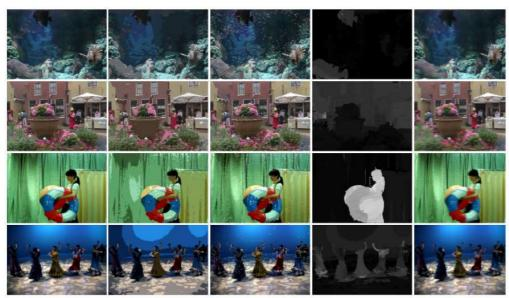
(a) Original image (b) Color segmentation (c) Feature selection (d) Motion estimation (e) Interlaced image
