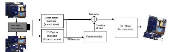
Fig. 1. Scene modeling system architecture
