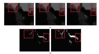
Fig. 6. (a) Up-sampled depth video of "Two men" obtained by 2D JBU and (b) difference images.
