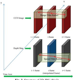
Fig. 3. Structure of 3D JBU (N=3).
