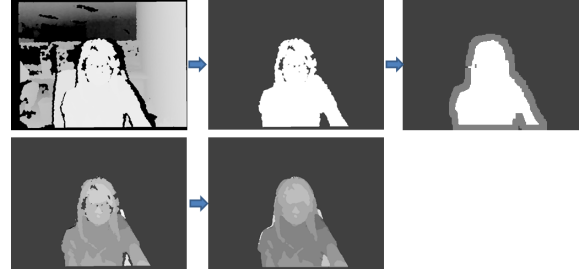
Fig. 3. Foreground segmentation and depth refinement are performed. Top: Input depth, initial foreground/binary map and trimap generation. Bottom: Initial depth map and refined depth image. Note that the contrast of the foreground depth map was enhanced for illustration purpose.
