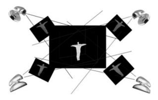
Figure 7. 3D modeling with a shape from silhouette and disparity.
