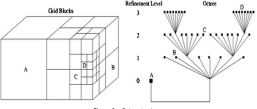
Figure 8. Octree structure.
