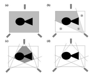
**Figure 6.** Shape from silhouette and disparity: (a) Whole volume containing objects; (b) Carving by the first camera; (c) Result by SFS; (d) Result by the proposed technique.
