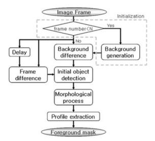
Figure 3. Block diagram of the proposed segmentation algorithm.
