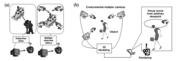
Figure 1. Capturing visual information: (a) Conventional approaches; (b) Proposed 3D video system.
