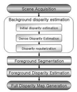
Figure 5. Block diagram of the fast disparity estimation algorithm.
