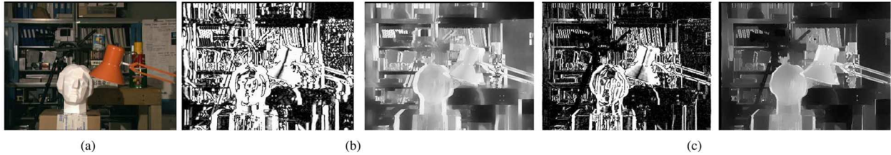
Fig. 1. Per-pixel and estimated costs in the “Tsukuba” image: (a) stereo image pairs, (b) per-pixel and estimated cost when disparity is 0, (c) per-pixel and estimated cost when disparity is 6. The estimated cost is computed with the proposed method, and \lambda is set to 1.0. We can find that the per-pixel cost is very noisy.
