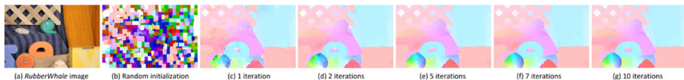
Fig. 6. After applying PMF for a few iterations, optical flow estimation for the RubberWhale images quickly converges.
