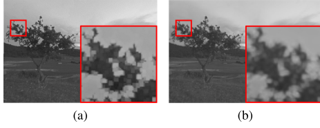
Fig. 3. Effect of the regularization term in Eq. (6). (a) initial illumination map with blocky artifacts. (b) predicted illumination map with L^{BCP} .
